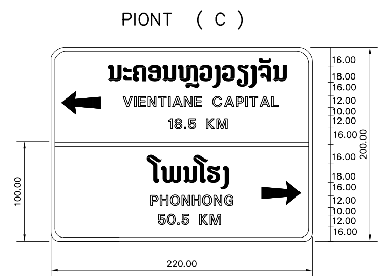
(NEW INSTALLATION) (FOR POST TYPE B)
