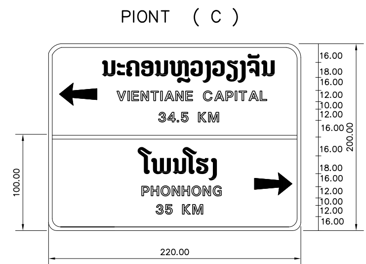
(NEW INSTALLATION) (FOR POST TYPE B)
