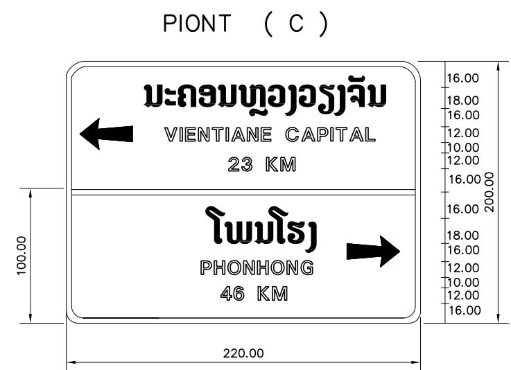
(NEW INSTALLATION) (FOR POST TYPE B)
