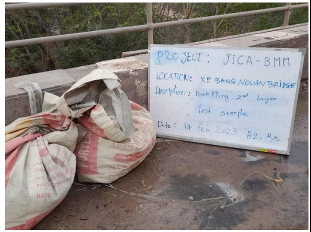
Backfilling by Soil cement 2 nd Layer on 14 th February 2023. Base course 5.0 m 3 + Portland Cement 500kg(Take a Test Sample)
