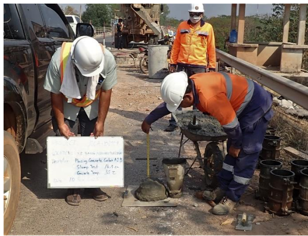
Concrete Casting for Concrete Corbel Abutment 1 Right side on 10 th February 2023. Slump test 16.5 cm, Concrete Temperature 35 °C
