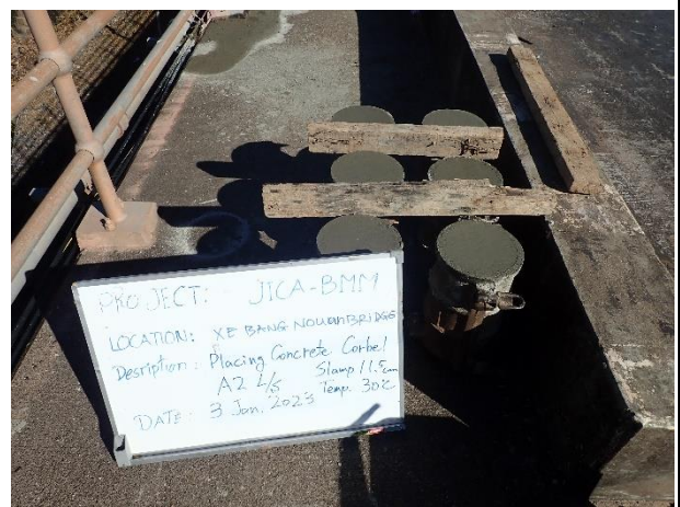
Concrete Casting for Concrete Corbel Abutment 2 Left side on 3 rd January 2023. Slump test 11.5 cm, Concrete Temperature 30 °C
