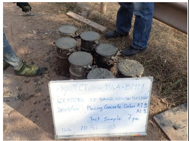
Concrete Casting for Concrete Corbel Abutment 1 Right side on 10 th February 2023. Slump test 16.5 cm, Concrete Temperature 35 °C
