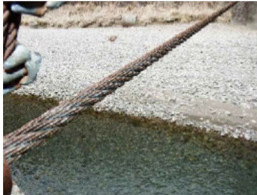
Rust preventive oil + Polyethylene coat
